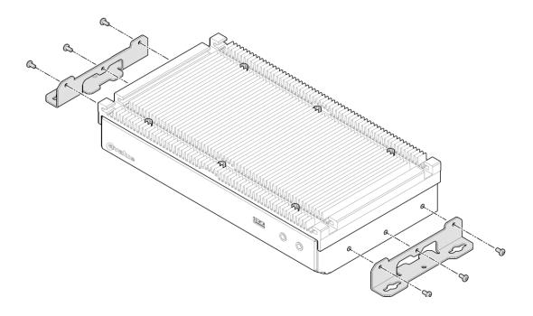
Step 1. Fasten 6 screws on both sides of ERS Rugged Embedded System.
