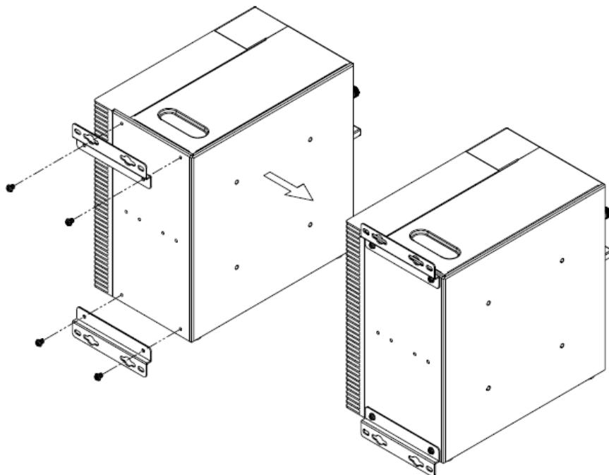
**Step1.** Position brackets on both sides, matching the holes on the system.
