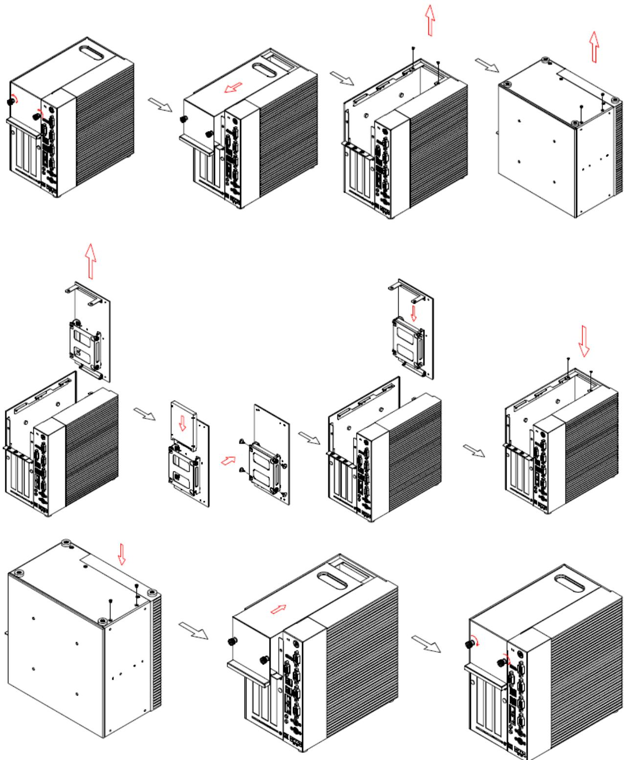
**Step1.** Remove 2 screws to release the cover.
