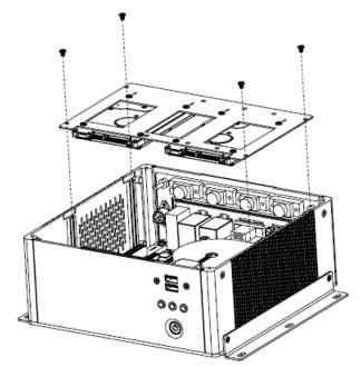
**Step2.** Remove 4 screws from the system to release the HDD bracket.
