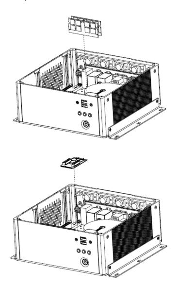
**Step4.** Slide the DDR4 SODIMM and Mini PCIE module into the sockets and press it down until properly seated.
