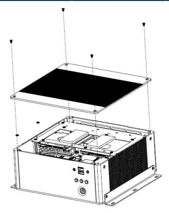
**Step1.** Remove 4 screws from rear side before removing back cover.
