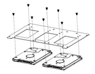
**Step3.** Secure 2.5" HDD/SSD by means of 8 screws.
