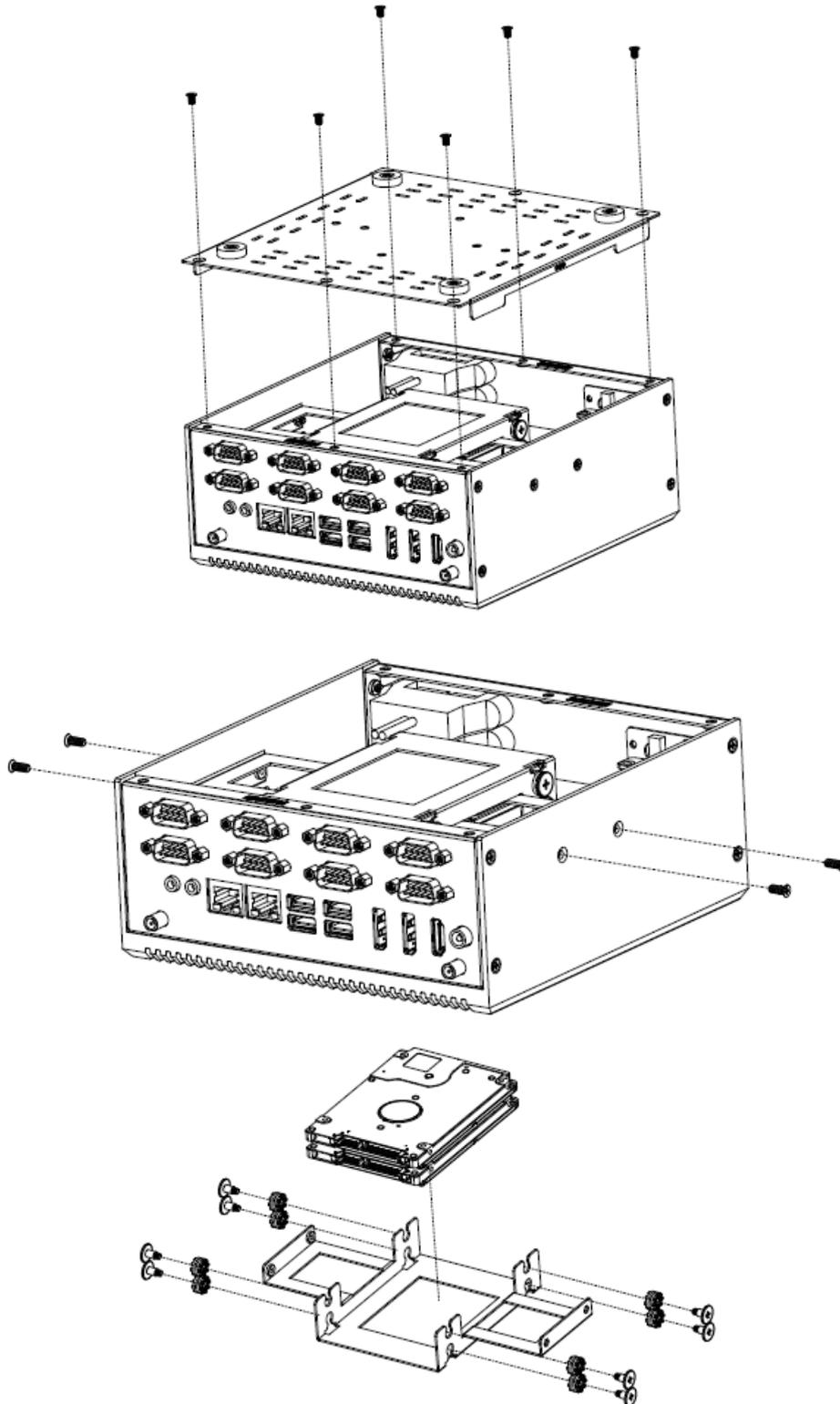
**Step1.** Remove 10 screws from rear and each side before removing back cover.
