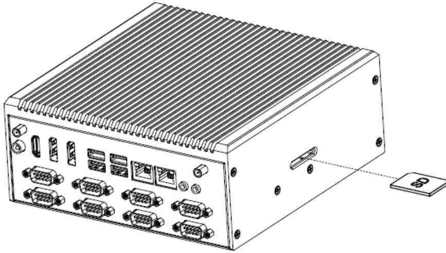
**Step1.** Insert SD card into SD slot.
